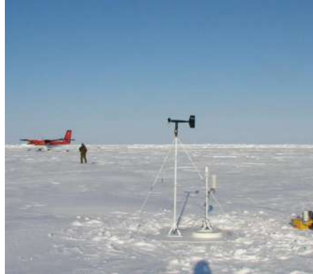
Fig. 1. Top: CALIB buoy dropped from Twinotter aircraft at 300 m altitude and descending on parachute. Bottom: PAWS buoy G after installation with Twinotter aircraft landed on ice.
